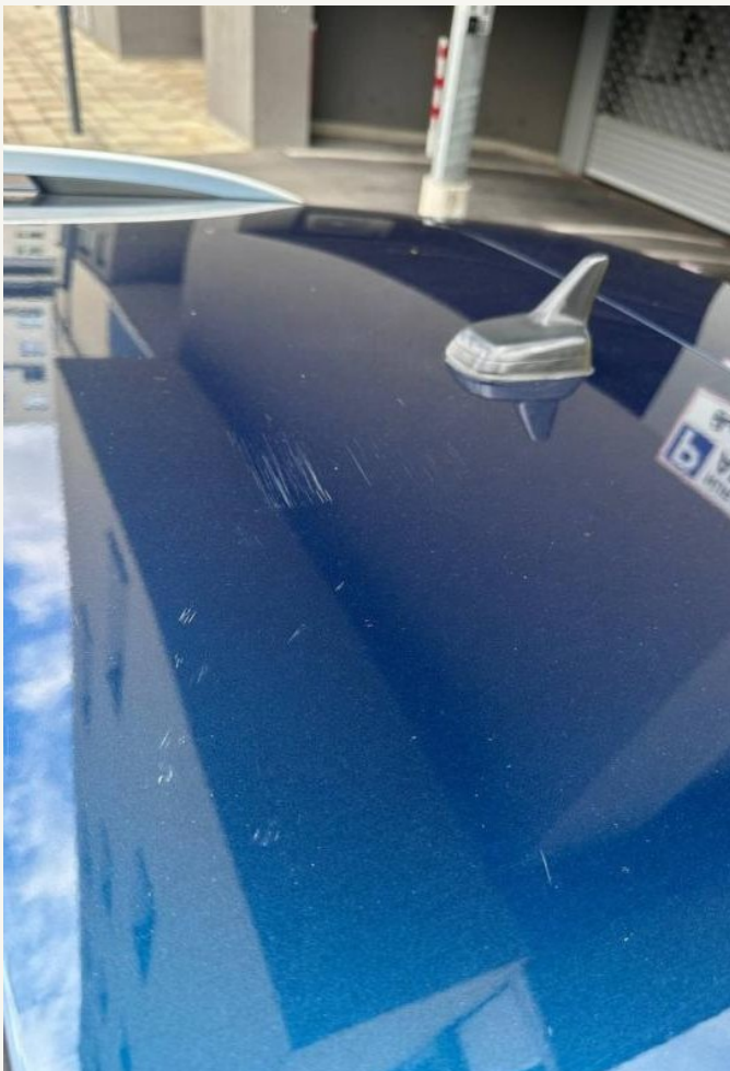
Wash/contact marks on roof
